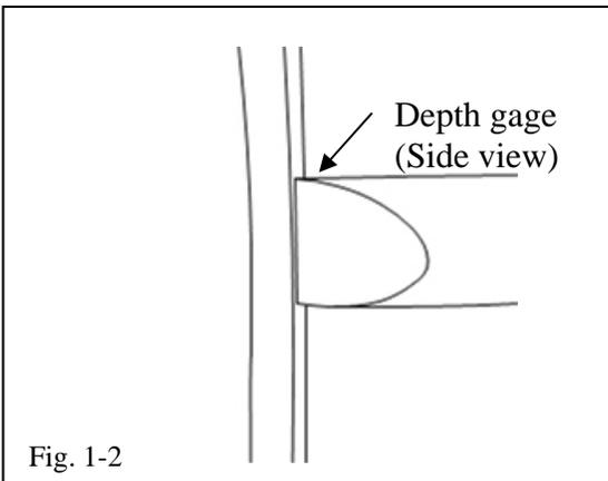
Align the adjustment tool to the edge of the door, with the angle edge positioned toward the inside of the door (Fig. 1-2).
